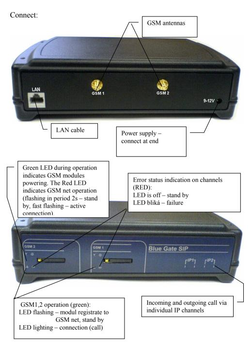
On PC connected to LAN from which you can control connected Gateway run various web broser. Insert IP adress of gate (default 192.168.1.250) and you can continue in parameters setting.
