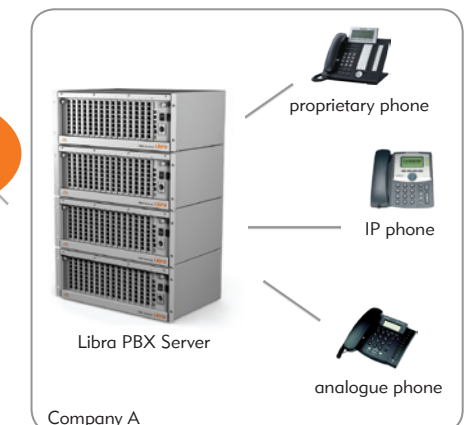
Platan Intelligent Networking (PIN) – intelligent networking of Libra servers using VoIP
