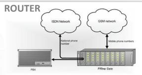
The gateway PRIma Gate is able to analyze dialed number and forward the call trough GSM Network or PSTN PRI access. Also, if all GSM modules are busy, it is possible to forward the call trough PSTN PRI network. Calls coming trough PSTN PRI access are forwarded directly to the PBX.
