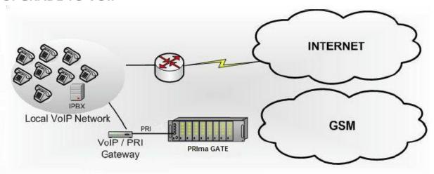
PRIma Gate can be integrated easily in VoIP structures connecting itself to a PRI/VoIP gateway.
