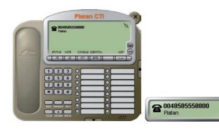
Information about the caller can be shown on the Platan CTI display, on a small notification window or on the Dispatcher console
